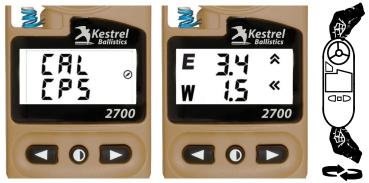
When calibrated, the display will change to show the solutions screen. **Note:** Every time the battery is replaced the compass in the 2700 will need to be recalibrated and the screen will display "CAL CPS".
